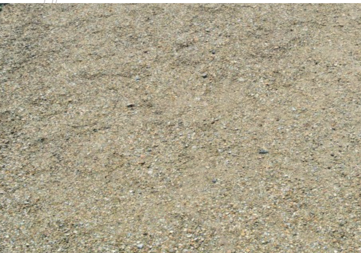
Struinpaden: halfverharding Maas mix (ecoDynamic)
